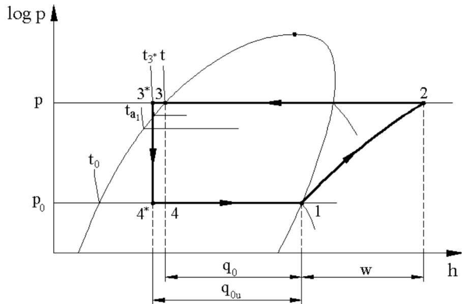
The sub-cooling in T-s and log p-h diagrams
