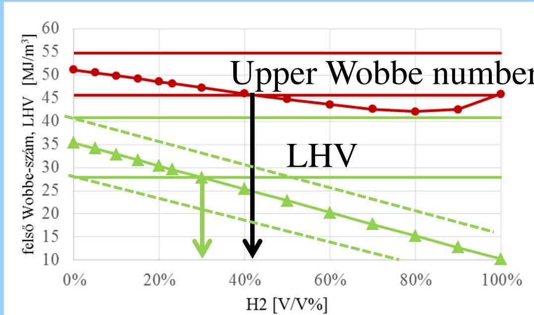
When hydrogen is mixed into NG, the calorific value (LHV) and Wobbe number of the mixture are removed from the prescribed ranges, However, how much mixing depends on the gas into which the hydrogen is mixed (LNG, interconnector network, etc.).
