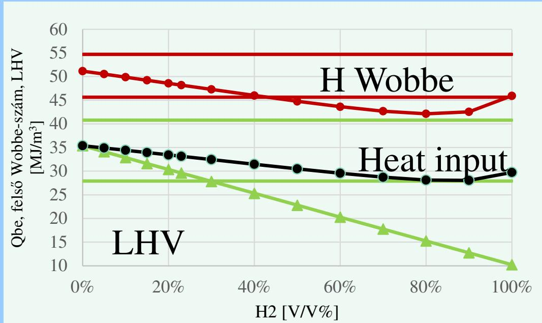
When mixing 20 V/V% H<sub>2</sub> into natural gas, the calorific value decreases to 86%, but the square root of density increases to 1.1%, so the theoretical flow rate increases, so the theoretically transferable heat decreases to only 95%!
