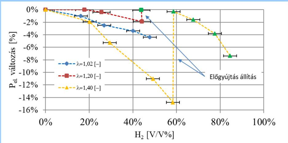
At a constant excess of air, the fuel flow rate increased by mixing H<sub>2</sub>, but performance and efficiency decreased
