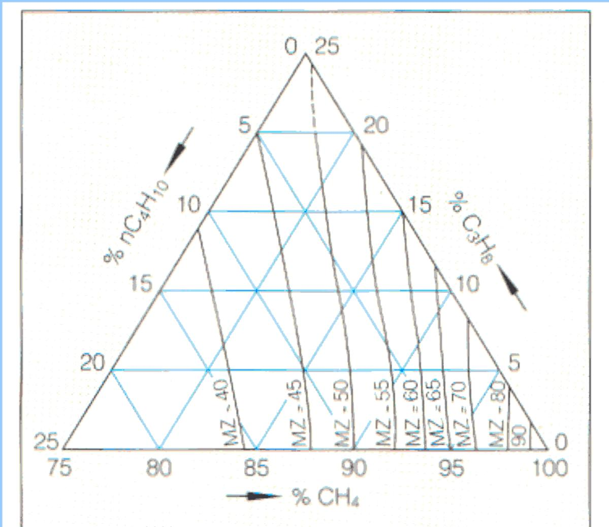
Fig. 17 Determining the methane number of the three-component mixture of methane/propane/butane
