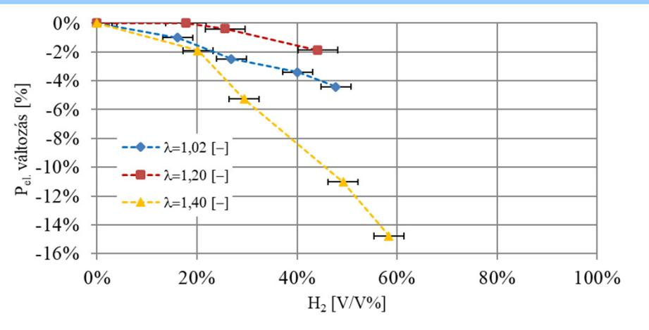
At a constant excess of air, the fuel flow rate increased by mixing H<sub>2</sub>, but performance and efficiency decreased
