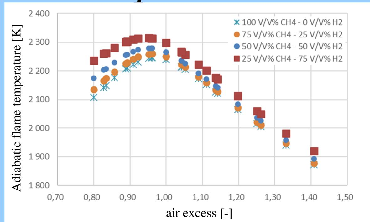
Adiabatic flame temperature as a function of air excess in case of different H<sub>2</sub> mixing (GRI 3.0 mechanism, T<sub>0</sub>= 323 K, P<sub>0</sub>= 0.1 Mpa)
